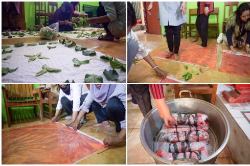
Figure 1. Steps for Ecoprint Batik Steaming Photocopy Method (Researcher's Documentation)
